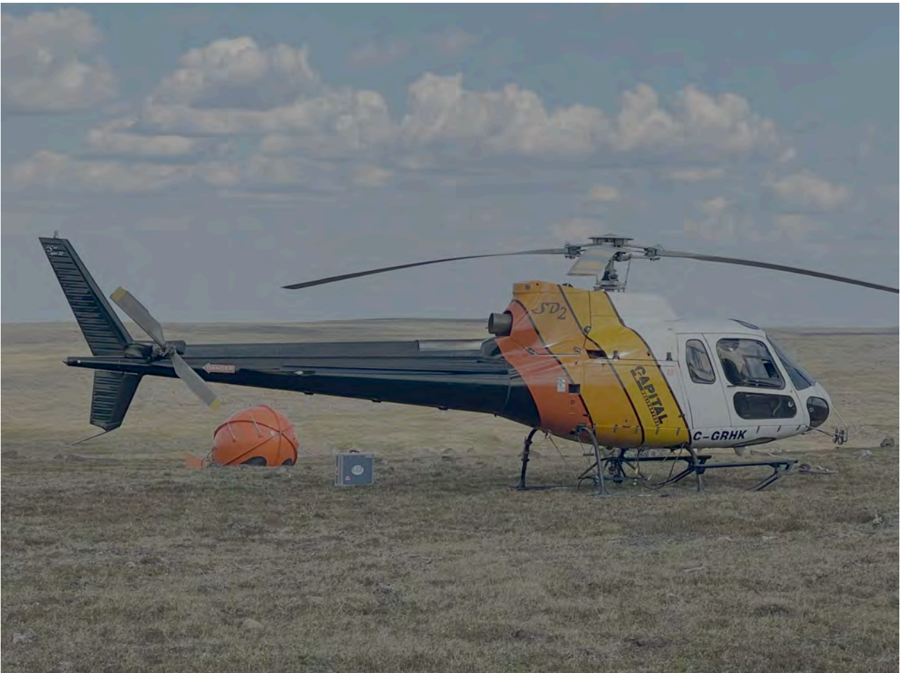
Figure 11: Expert Geophysics latest generation MobileMT airborne electromagnetic survey equipment in action at Rae Cu-Ag project
