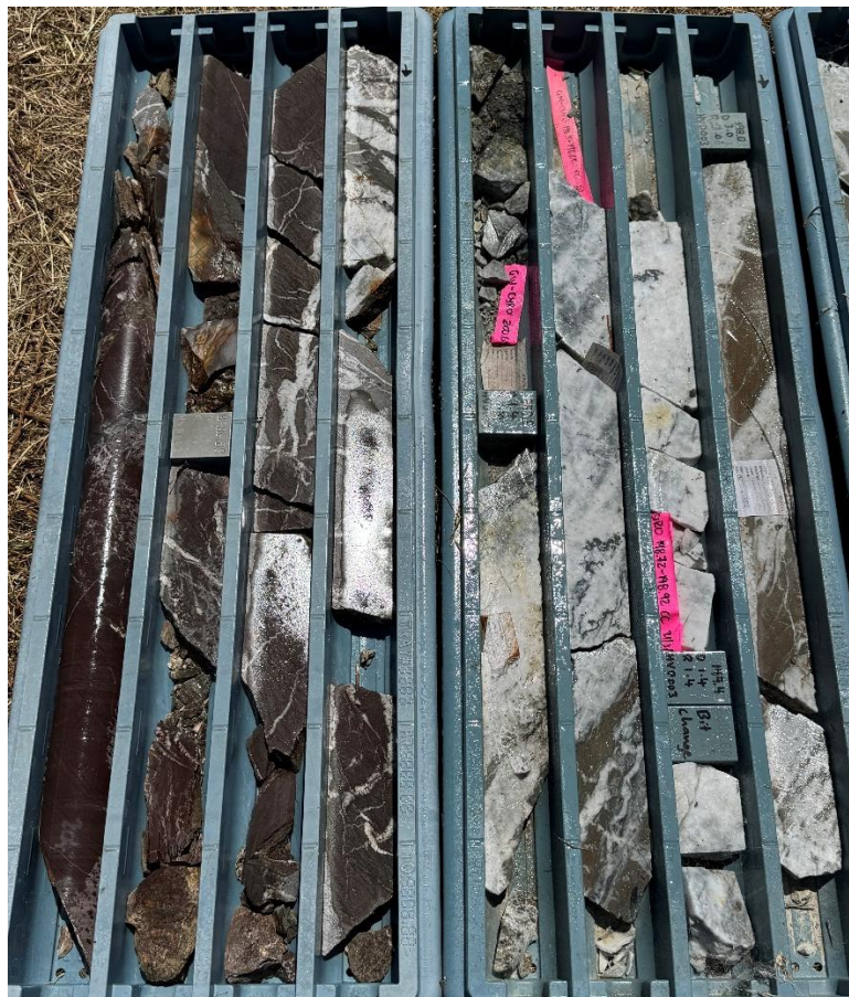
Figure 5. Photo of previously drilled core from hole HVD003 (~198-203m down hole) at the Happy Valley Trend showing quartz veining (white) that hosts the high grade mineralisation. This core forms part of an interval that graded 11.5 metres at 160.4g/t Au . Full details of the previous drilling can be found in the Advance Metals' ASX release dated 6 January 2025.
