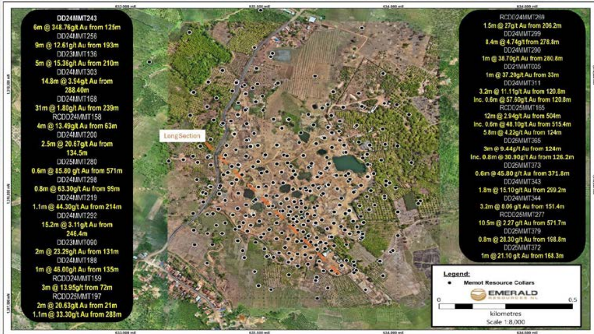
Figure 28 | Memot drill collars and significant intercepts
