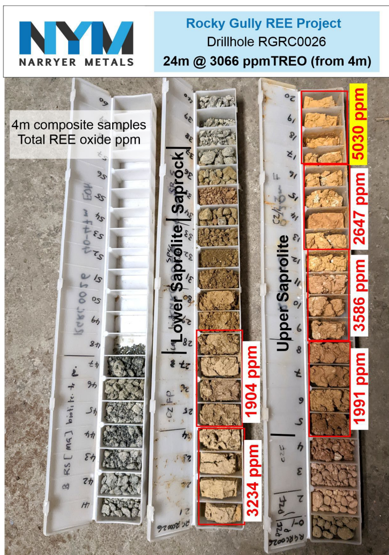
Figure 5. Total rare earth oxide 4m composited grades in clay host seen in chip trays from drillhole RGRC026, Ivar Prospect
