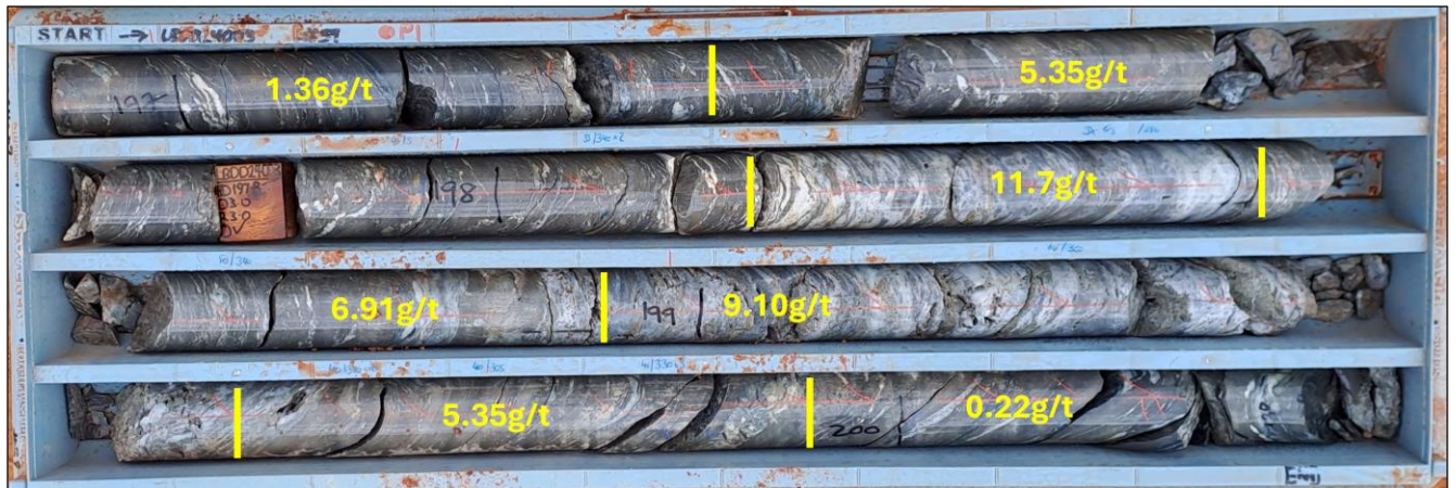
Figure 5 - Core photo from drillhole LBDD24003, showing one of the high-grade zones (1.36m @ 9.23g/t from 198.21m) within an overall intercept of 20.39m @ 3.03g/t from 196.53m
