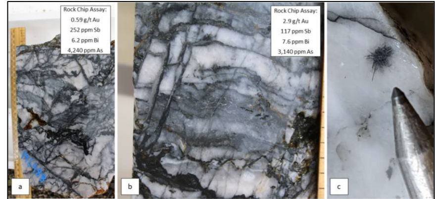
South Muckleford rock chip samples collected from the Fentiman's Reef historic mine waste dump: (a) mineralised quartz vein with abundant stylonite and breccia textures; (b) disseminated sulphides (arsenopyrite, stibnite and pyrite) within a stylonitic and brecciated quartz vein; and (c) coarse stibnite ( \text{Sb}_2\text{S}_3 ) crystals and thin stylonites within a mineralised quartz vein 20
