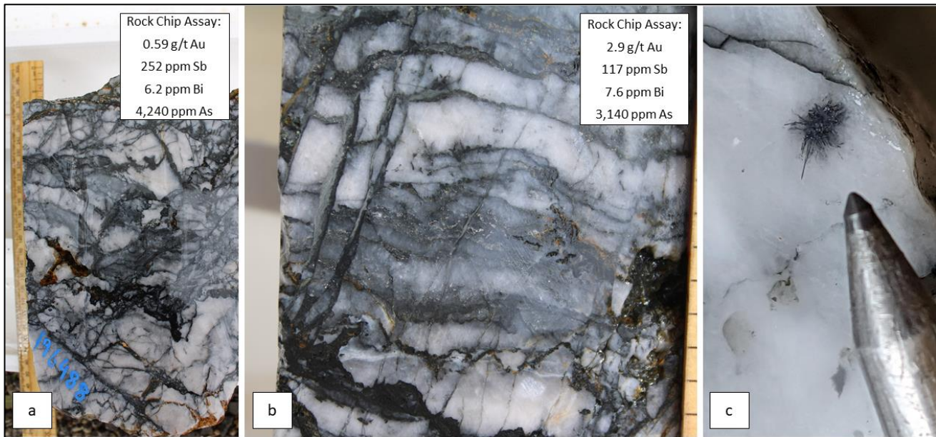
Figure 4: Rock samples collected from the Fentiman’s South historic mine waste dump: (a) mineralised quartz vein with abundant stylonite and breccia textures; (b) disseminated sulphides (arsenopyrite, stibnite and pyrite) within a stylonitic and brecciated quartz vein; and (c) coarse stibnite ( Sb_2S_3 ) crystals and thin stylonites within a mineralised quartz vein. Scale ruler in Figure 4a. 3
