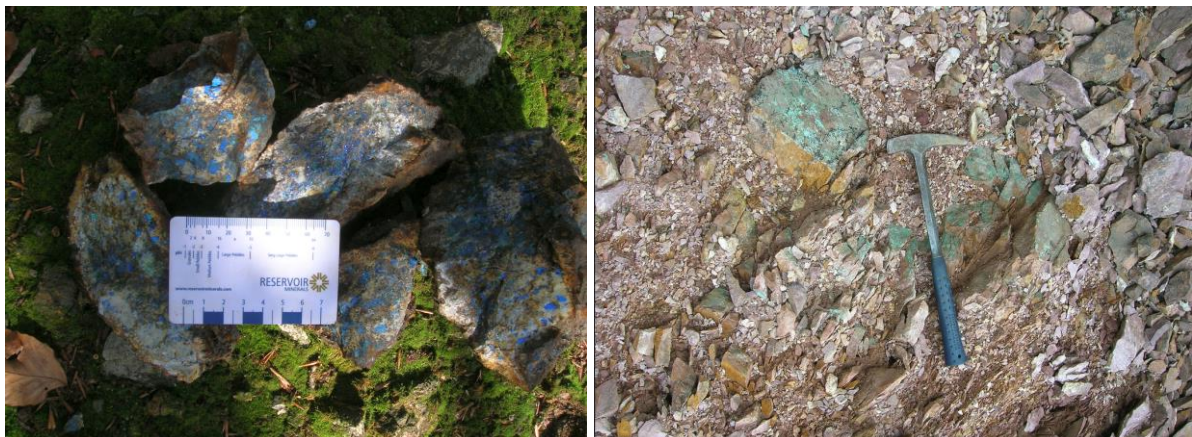
Figure 5b – Mineralised Jurassic limestone at Kopajska Reka with 5-15% disseminated azurite (Sample KP1) (LHS) and altered Permian Sandstone with malachite at Gradac (Sample REG-104920 1.3% Cu) (RHS) – refer Appendix 1.
