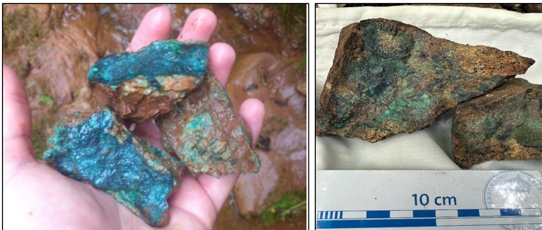
Figure 1 - Sample REG-104923: 20% Cu and 1540ppm – displaying massive chalcocite, azurite and malachite (LHS) and ST008: 6.5% Cu and 155ppm Ag displaying malachite and azurite in sandstone (RHS) (refer Appendix 1)
