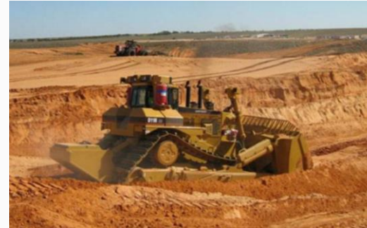
Image: Typical dozer push operation
