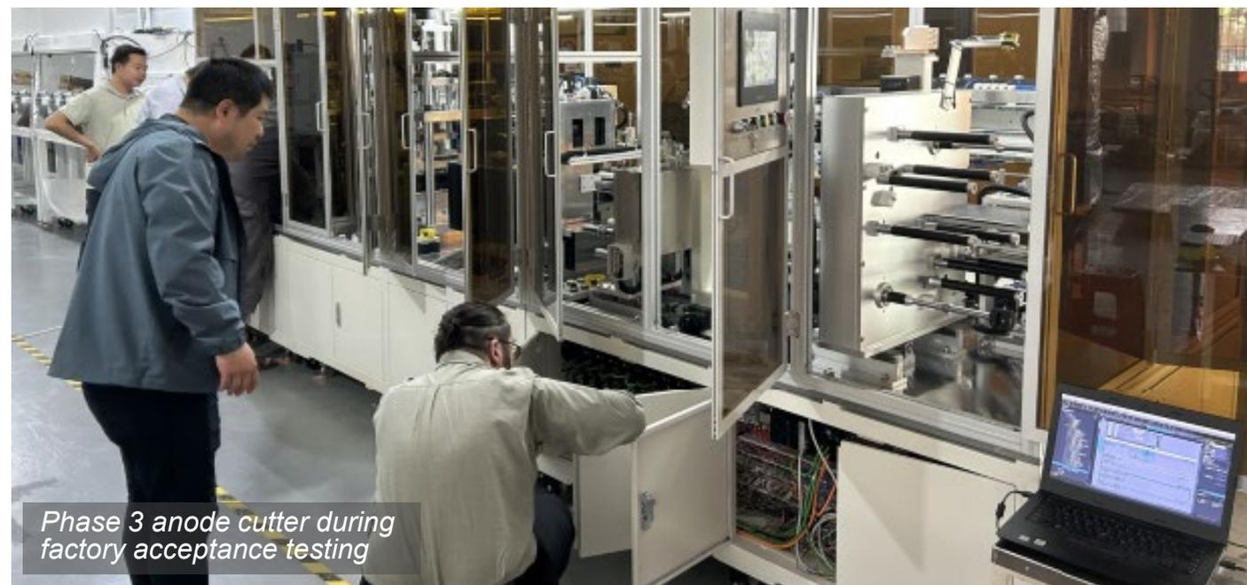
*Phase 3 anode cutter during factory acceptance testing*
