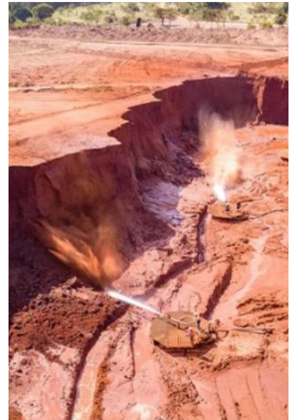
Image: Example mineral sands hydraulic mining operation Reference: Image of Base Resources Ltd, Kwale Operation, Kenya
