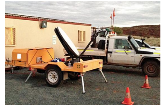
Image: Example of a mine site VSAT system for remote site communications
