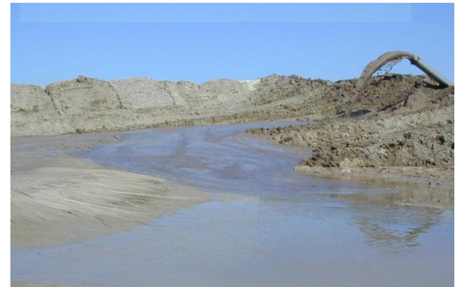
Image: Flocculated Co-disposal of Sand Tails and Slimes
