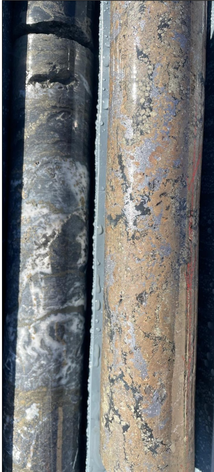
Figure 16: 26DDBR007 massive sulfide zone, sphalerite (brown), galena (metallic), pyrite (bronze cubes) from 242.1m to 242.4m.
