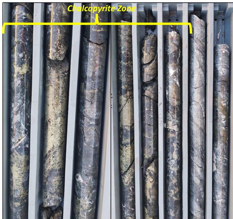
Figure 1: Semi-massive copper-bearing mineral chalcopyrite (yellow) and sphalerite (brown), in 26DDBR006 from 361.5m to 368.0m.
