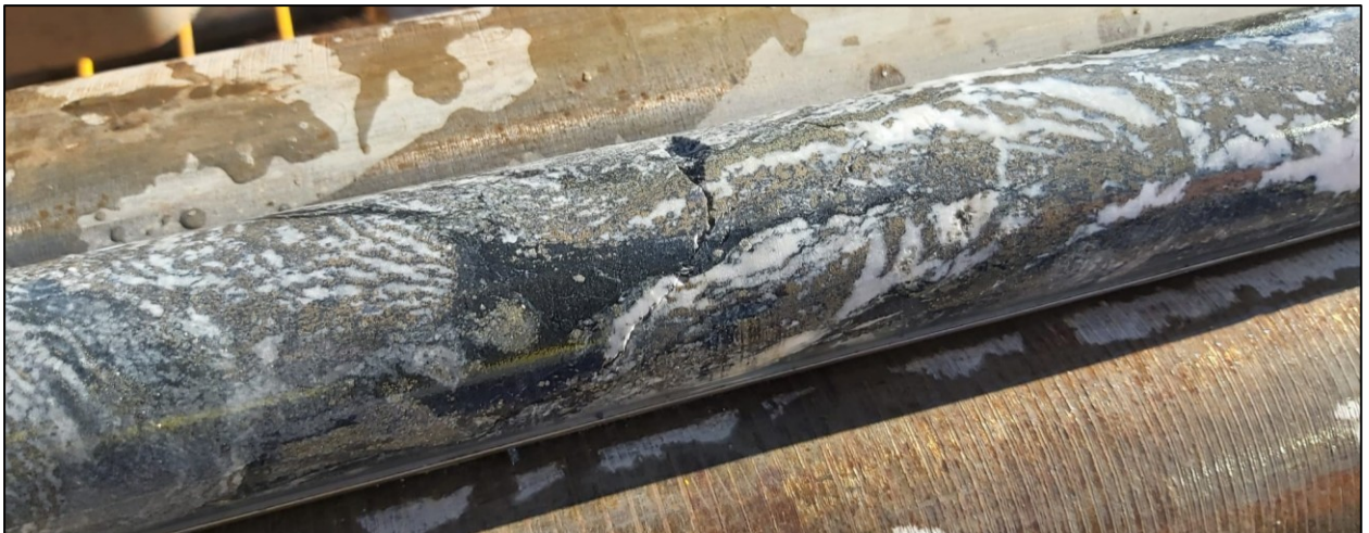
Figure 9: 26DDBR002 banded and semi-massive sulfides, dominantly sphalerite, galena and pyrite, replacing a marl, 323.7-324.0m.
