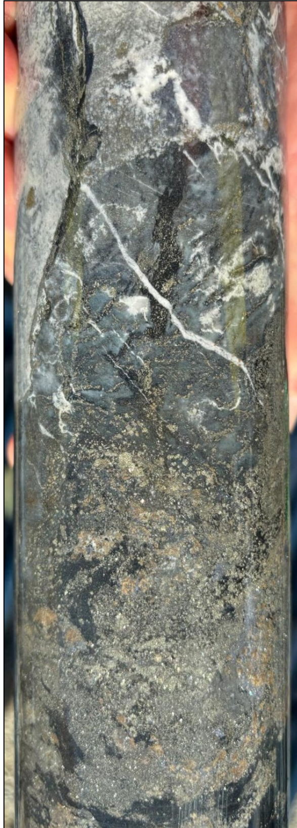
Figure 14: 26DDBR004 semi-massive pyrite (bronze) and lesser sphalerite (Brown) 197.2 - 197.4m
