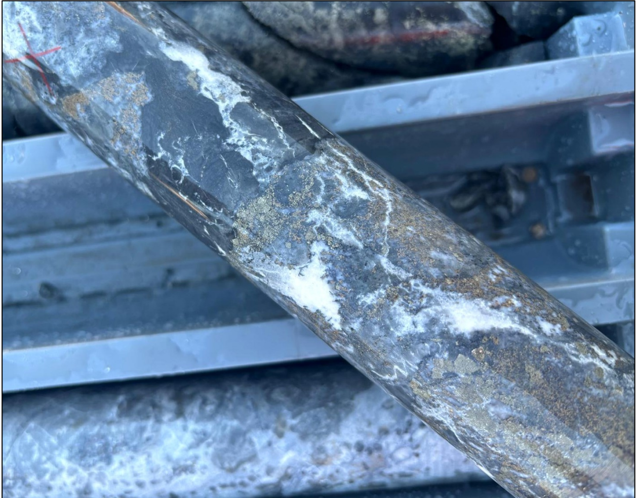
Figure 4: Footwall quartz-carbonate alteration with sphalerite-pyrite (brown-bronze) immediately below the chalcopyrite zone in 26DDBR006 from 368.5 to 368.7m.
