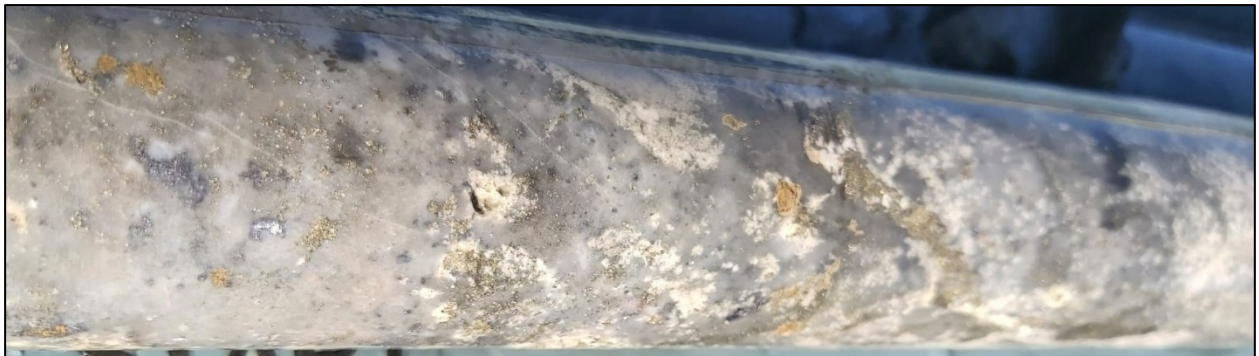
Figure 11: 26DDBR003 footwall pervasive quartz alteration with 5% disseminated galena, sphalerite and pyrite 363.6 - 363.8m.
