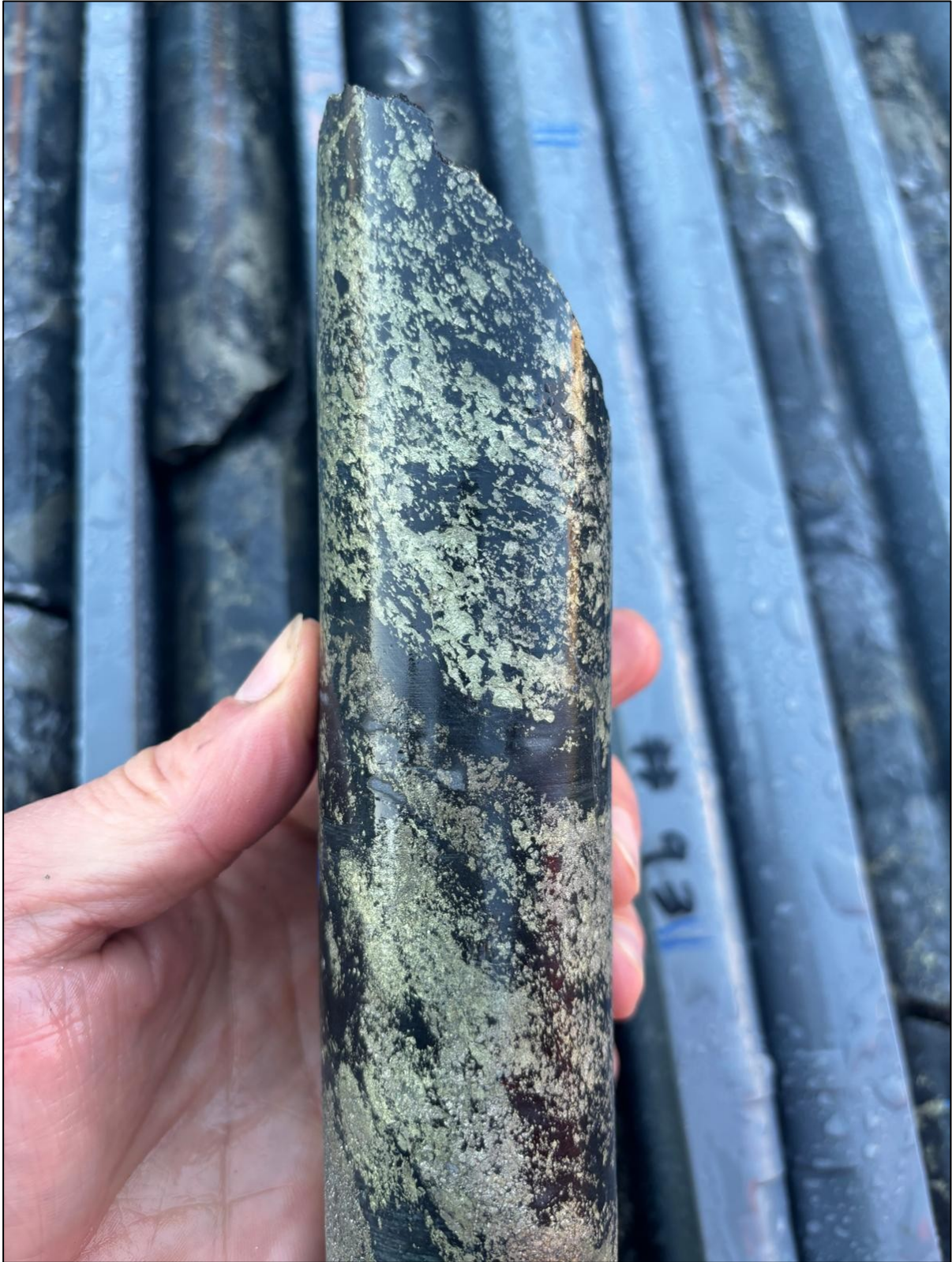
Figure 2: Core photograph of 26DDBR006 with semi-massive chalcopyrite (yellow) and pyrite (bronze). Core interval from 366.6 to 366.8m.
