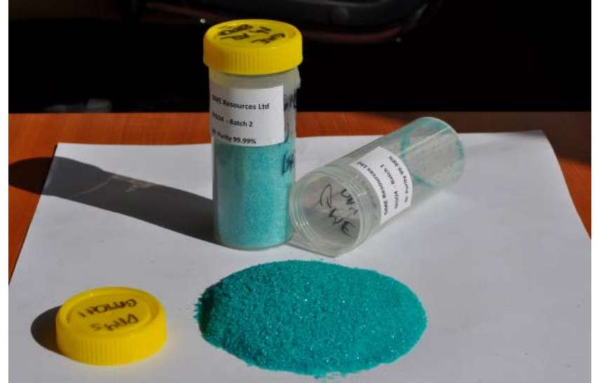
Nickel sulphate produced from NiWest ore through GME's metallurgical test work program
