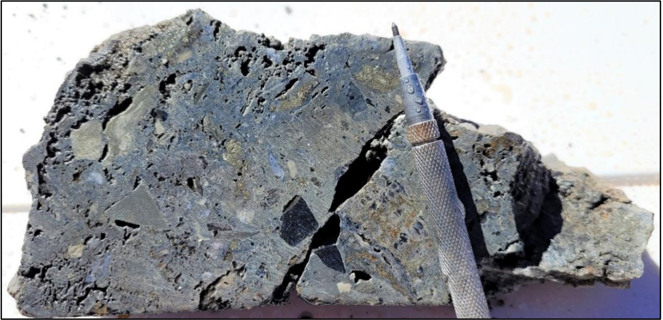
Photo 5 - PQ3 half core collected at 121m from EHD034 showing coarse grained sphalerite, pyrite, and galena hosted within the Navajoh Unconformity Unit. Note: core diameter is 83mm
