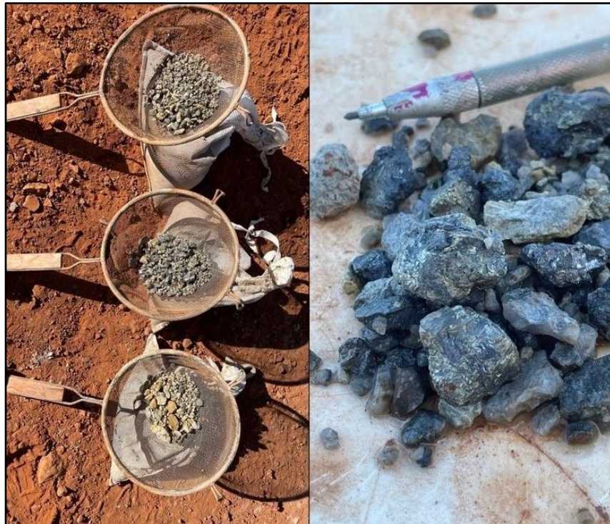
Photo 2 & 3 – EHRC720 sieved Unconformity Unit and sulphide examples. Left: EHRC720 sieved unconformity unit host lithology chips from 161-164m. Right: EHRC720 Select sieved sulphide bearing samples from interval 162-163m showing coarse sphalerite, galena, and pyrite. Refer to Table 2 for further observations.
