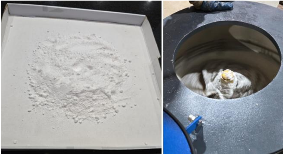
Figure 7: 98.9% Lithium Carbonate (left) and processing in the plant's centrifuge (right)
