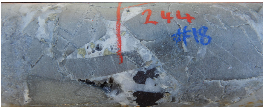
Hydrothermal infill breccia CAE hole # 18, : 244m depth. Grey hornfels clasts , infill white calcite, clear quartz, brassy pyrite, black sphalerite. Interval 244m-245m : 1m @ 3.99 g/t Au, 0.24% Cu ,16.1 g/t Ag.
