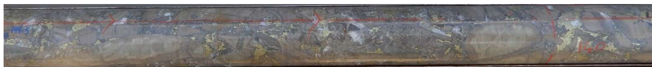
Fig 11 Full HQ Core. Copper rich hydrothermal infill breccia ,140m, with clasts hornfels, infill chalcopyrite , pyrite, quartz ,calcite, minor chlorite. 139m-140m returned 1m @ 4.43% CuEq%, 3.73% Cu,0.64 g/t Au,38 g/t Ag, 6.37% S.
