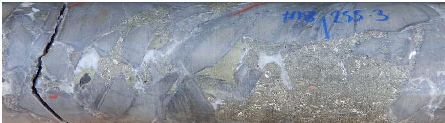
High grade gold section of sulphidic hydrothermal infill breccia CAE hole# 18, 255.3m. Interval 255m-256m : 1m @ 22.93g/t Au ,0.61 g/t Au, 61.0 g/t Ag with elevated Zn.
