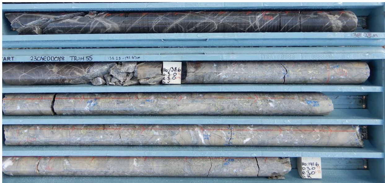
Fig 10 Contact at 138. 6m of flinty hornfels uphole and hydrothermal infill breccia (downhole) dominated by angular hornfels clasts with calcite-quartz-pyrite-chalcopyrite infill. Full HQ core, Hole 18 :138m-142m returned 4m @ 1.79g/t CuEq%,1.50 % Cu,0.25 g/t Au,16.6 g/t Ag
