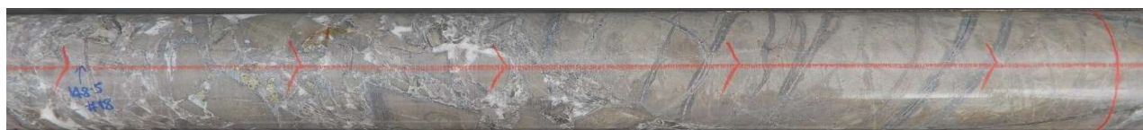
Fig 12.Full HQ Core : Hydrothermal breccia 148.5m,dominated by clasts hornfels, infill quartz ,calcite, minor pyrite, chalcopyrite . Clasts are extensively cut by thin porphyry style pyrite veins with quartz sericite alteration selvages. 148m-149m: 1m @ 0.35% Cu,0.04 g/t Au,4.3 g/t Ag, 1.77% S.
