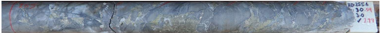
High grade gold section of sulphidic hydrothermal infill breccia CAE hole# 18, Interval 255m-256m : 1m @ 22.93g/t Au ,0.61 g/t Au,61.0 g/t Ag with elevated Zn
